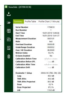
A number of default view configurations are provided to rapidly configure NoiseSafe to suit noise exposure assessment methods as defined by local or international standards (e.g. **ISO9612**). To provide a good starting and we recommended you load a view configuration as appropriate to your assessment protocol, this can be adjusted to meet your exact needs and then saved for future use.
