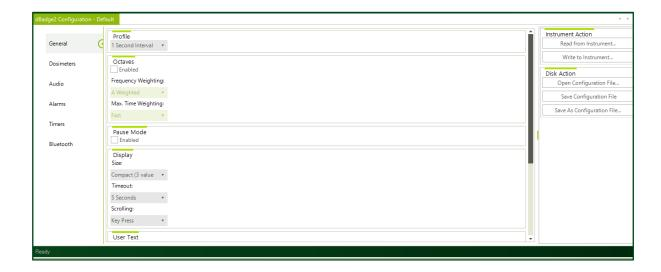
To Open a Saved or Default dBadge2 Instrument configuration, select 'Open Configuration File' from the Disk Actions list.
