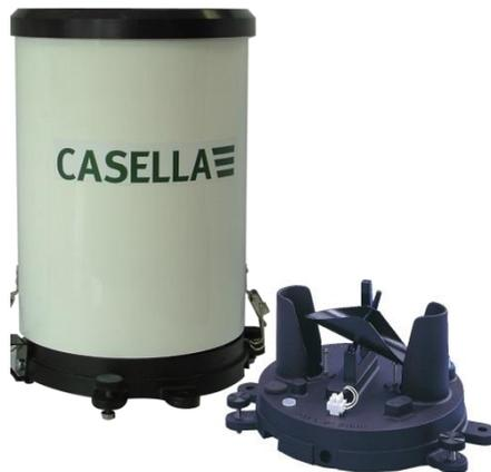
Figure 1: The Tipping bucket rain gauge with the outer cover removed.
